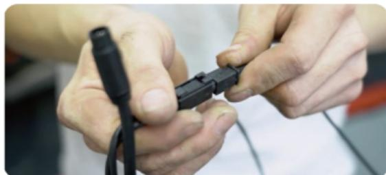
Please avoid bending the F1 camera cable at a sharp angle, as bending it at a sharp angle can damage its shielding and cause improper signal transmission or interference with other electronic devices.
