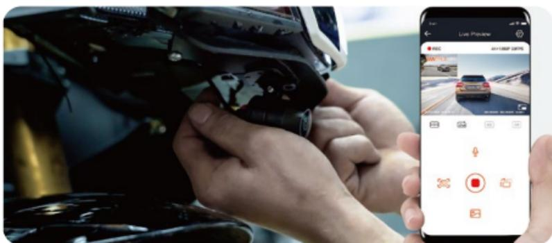
After the camera is installed, you can enter the VANTRU App real-time preview to correct the camera orientation. After entering the live preview, click on the word [田] calibration line at the bottom left of the screen to confirm the camera direction.
